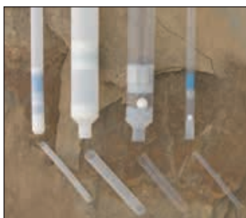
Polyethylene bailers are opaque; PVC and FEP bailers are clear.
