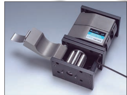
Stack heads for up to 32 channels.
