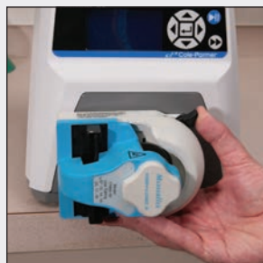
1. With head on drive, rotate activator lever counter-clockwise to open occlusion bed and tubing retainers.
