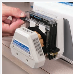
3. Adjust occlusion using index scale on cartridge.
