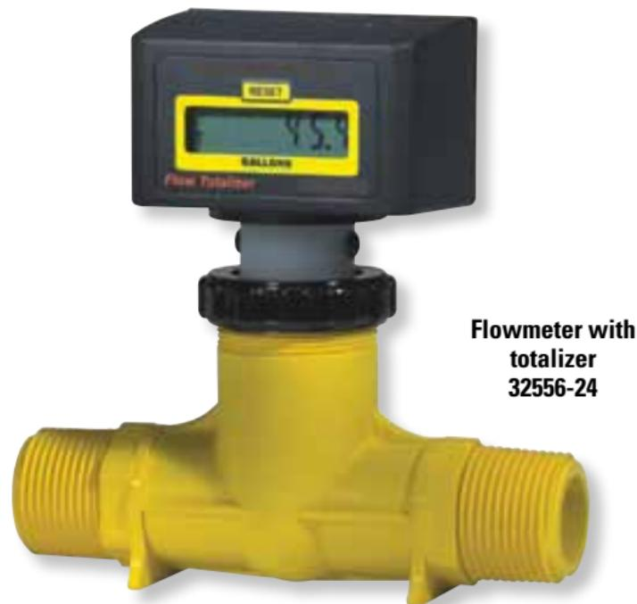
These injection-molded in-line flowmeters are battery powered (two AAA batteries included) making them perfect for remote locations. Enclosure is rated NEMA 4X and can be used in outdoor locations. Sensor is constructed of corrosion-resistant PVDF; in-line NPT(M) fittings are of PP.
