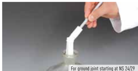
For ground joint starting at NS 24/29
