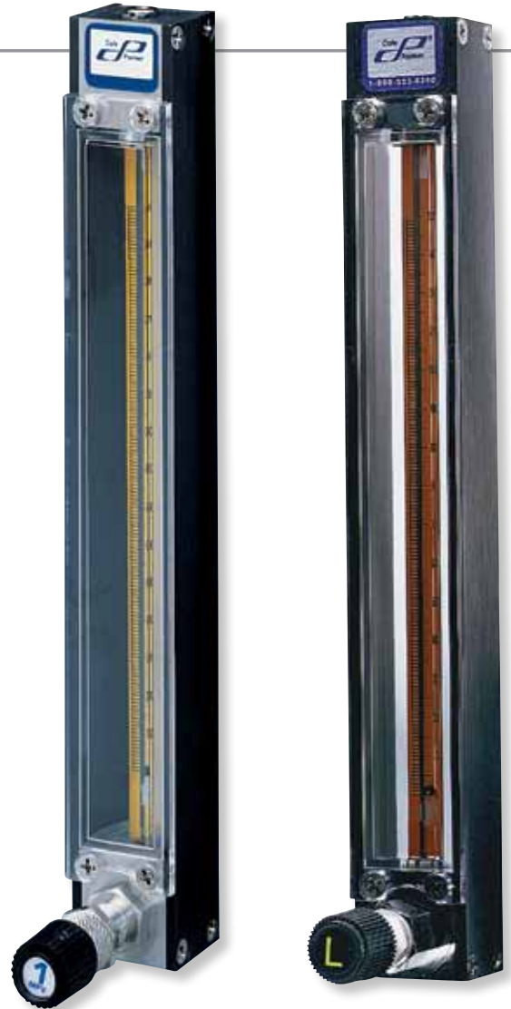
Brass flowmeter 03294-16 with valve
