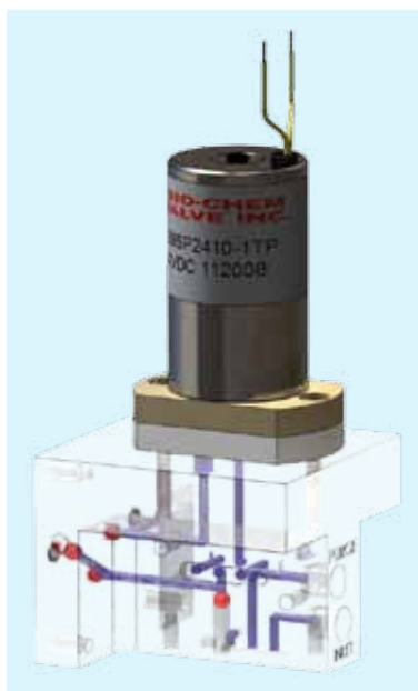
Custom manifold for (1) 139SP Micro-Pump (shown) and (3) isolation valves (not shown). Blue lines indicate the fluid path; the red dots are ruby balls used as plugs.
