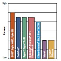
All tubing types accept pressure, but the firmer formulations accept more pressure than the softer types of tubing.
