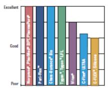
Vacuum/suction lift capability depends greatly on the tubing's ability to maintain its shape. Thus, a firmer tubing type in the smallest possible bore size will generate a stronger vacuum for your application. Higher drive speeds are required to generate the strongest possible vacuum with some tubing sizes.
