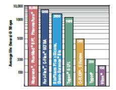
The graph above displays the average tubing life in hours of Masterflex® tubing. This tubing was tested in a Masterflex® pump head continuously pumping water at 70°F (21°C) and 0 psig (0 bar). Tubing life is calculated to time of failure or of 50% reduction in flow rate, whichever comes first. Reduce drive speeds to extend tubing life. Average tubing life for L/S® 16, I/P® 73, and B/T® 91 tubing at various speeds are listed in the table below.
