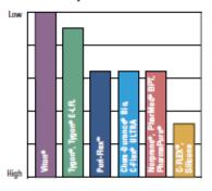
To minimize permeation of gases through the tubing wall, use firm tubing. Masterflex<sup>®</sup> L/S<sup>®</sup> and I/P<sup>®</sup> High-Performance precision tubing (L/S<sup>®</sup> 15, L/S<sup>®</sup> 24, L/S<sup>®</sup> 35, L/S<sup>®</sup> 36, I/P<sup>®</sup> 70, I/P<sup>®</sup> 88, and I/P<sup>®</sup> 89) is less permeable than Precision tubing sizes.
