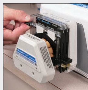
3. Adjust occlusion using index scale on cartridge.
