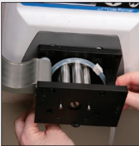
1. Release latch and open occlusion bed; place tubing over rollers and thread ends through retainer slots.
