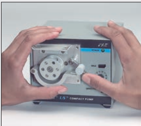
1. Release occlusion bed latch and open occlusion bed.
