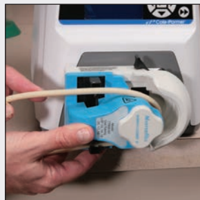
2. Place tubing over rollers and through retainers.
