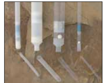
Polyethylene bailers are opaque; PVC and FEP bailers are clear.
