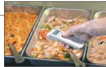
TempTestr 35625-15 eliminates interference from steam.
